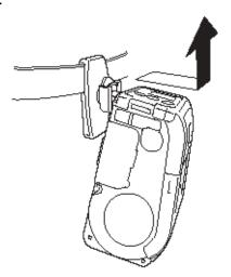
Pull the printer sideways and upwards to remove it from the belt hook.
